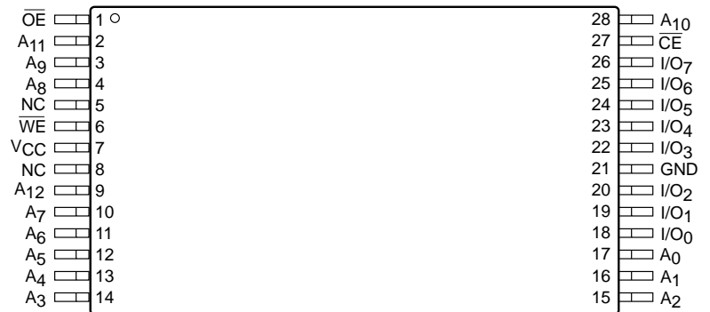
TSOP Top View (8mm x 13.4mm) (H13)
